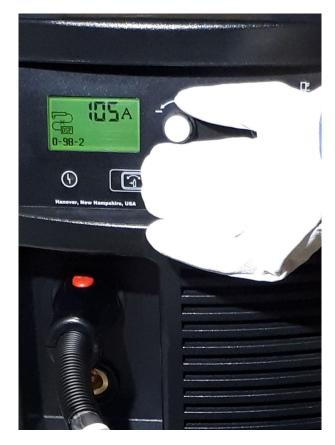
The ALARM switches off automatically by turning the potentiometer on the front of the machine.
