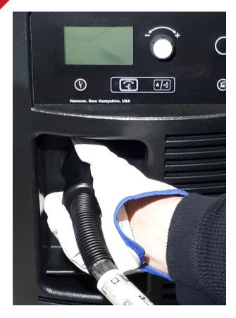
TURN OFF the generator. Connect the torch to the generator.
